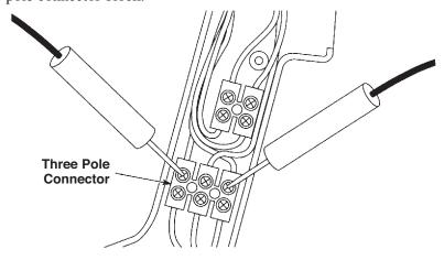
17. If no continuity exists, replace on/off switch assembly 62-9895-0024-4. If continuity exists, proceed to next step.
