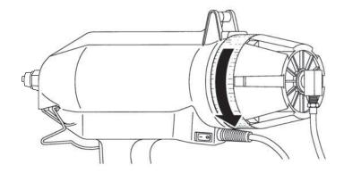
3. Inspect inside of end cap for improperly seated or damaged seal. Reposition or replace seal if necessary with end cap seal 62-9895-0004-6. If this does not produce adhesive flow, proceed to next step.
