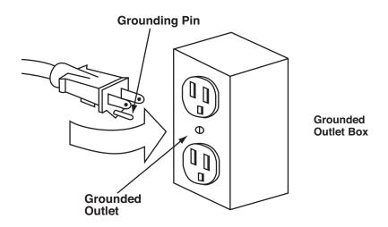
The Scotch-Weld PUR Easy Adhesive Applicator is intended for use on a nominal 120-volt circuit and has a grounding plug as shown in the figure above. Make sure the applicator is connected to an outlet having the same configurations as the plug. Do not use an adapter.
