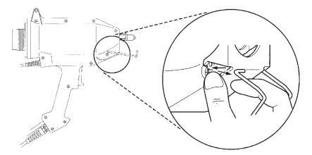
Remove end cap by turning counterclockwise.
