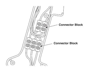
14. Use volt/ohm meter to check the heat tube assembly. Place one probe in upper left position of two pole connector blocks. With the other meter probe, touch the connector on upper right side of two pole connector.
