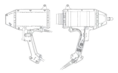
13. Inspect all wire connections for loose or disconnected wires by making certain screws in all connector blocks are securing the wires properly. If any connections are loose and have pulled out of connector blocks, reconnect and tighten connection per wiring diagram.
