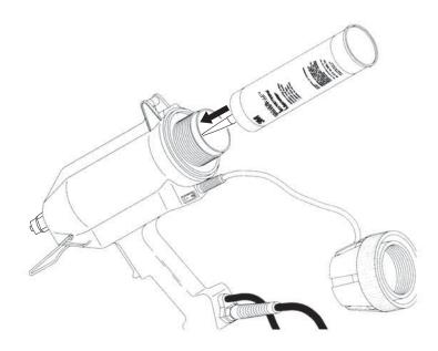
6. Adjust the Shroud: With a Scotch-Weld PUR Easy adhesive cartridge and Disposable Nozzle loaded in the applicator, insert Nozzle Shroud (A) into Nozzle Warmer (B) allowing Approximately 1/16" of the Disposable Nozzle protruding as shown and tighten set-screw (C) to secure
