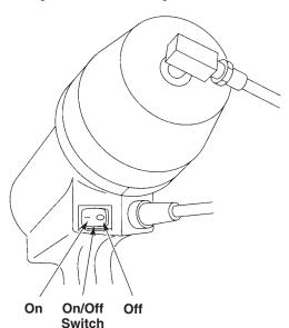
Remove power cord from grounded electrical outlet and disconnect air supply before conducting any further evaluations or repairs.
