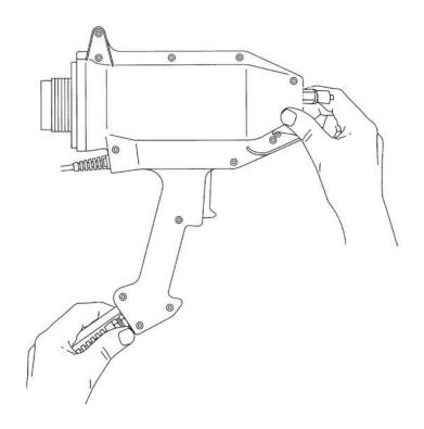
18. Hold the trigger in the upper housing and lift off.
